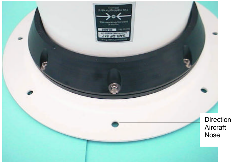
Fig. 2-5 Montage direction of the antenna unit
